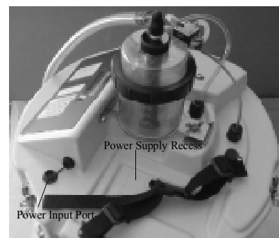
Top of VST showing power supply recess
